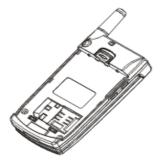
Slide the SIM card into the slot with care.
